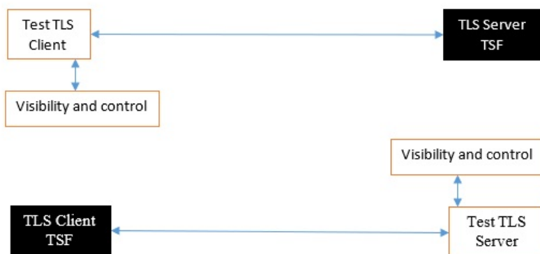
Figure 2: Test environment for TLS 1.3 using custom endpoint capabilities for visibility and control
